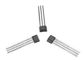
The SS490 Series MRL (Miniature Ratiometric Linear) sensors are small, versatile linear Hall effect devices which are operated by the magnetic field from a permanent magnet or an electromagnet. The ratiometric output voltage is set by the supply voltage and varies in proportion to the strength of the magnetic field.
