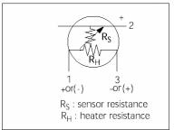
Fig 1c. Equivalent circuit
