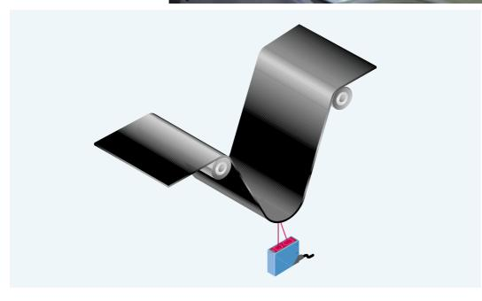
$\blacktriangleleft$  In continuous tyre production, supply loops regulate web tension and, therefore, the tensile force in the material. The WTA 24 ensures that the loops are fed evenly.
