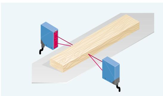
■ On circular crosscut saws, the width is measured continuously while the boards are automatically advanced. WTA 24 sensors see to this reliably.
